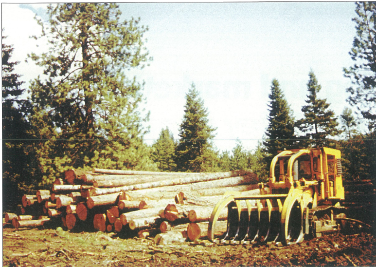
Figure 53.— Ponderosa pine should be felled, bucked, skidded, and delivered to the mill as quickly as possible to avoid blue stain problems.
